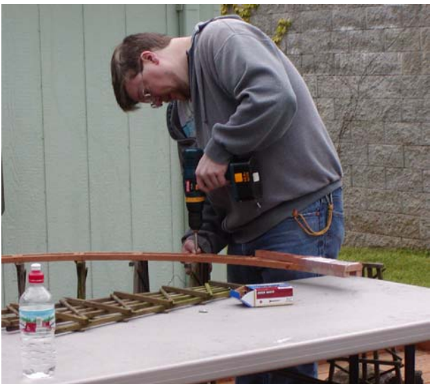
Dave Stratton anchors the roadbed to one of the trestles.
